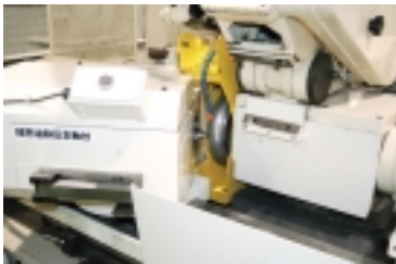
Corrective grinding on the center with a high-precision hydrostatic workhead (roundness at 0.2 \mu\text{m} )
