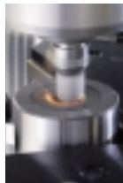
SHIGIYA developed ultra-precision center hole grinder aims for roundness at 0.1 \mu\text{m} of wheel spindle.
