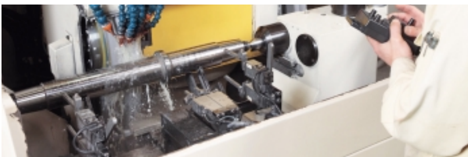
CNC universal grinder that grinds at a roundness of 0.1 \mu\text{m} with wheel spindles that are the core of cylindrical grinders.
