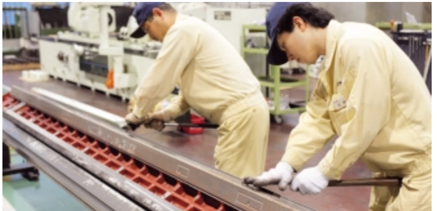
Scraping work for sliding surfaces
