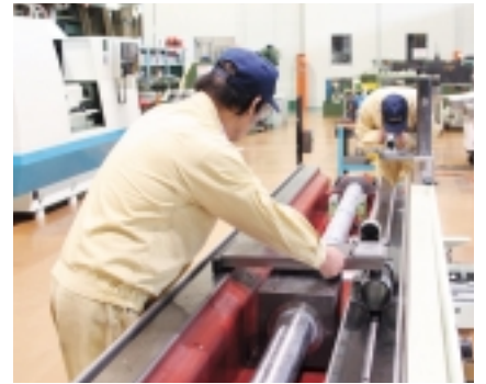
Measuring the straightness with an autocollimator
