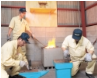
An in-house fire pit installed for man-made scrapers
