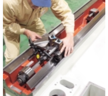
Centering for ball screw attachment
